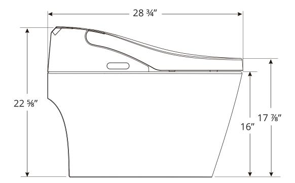
**ATTENTION!** Dimensions may vary by up to 3/8". It is highly recommended to pull all dimensions of actual model for installation and measuring purposes.
